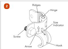
With the screw loosened fold out the outer part of the Eyedog.
