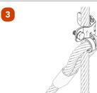
Apply the Eyedog on the lifting part of the wire making sure that the arrow on the Eyedog is pointing upwards, i.e. in the direction of the loose sling wire end towards the crane hook or other lifting device.
