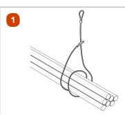
Apply the sling as normal by wrapping the sling twice around the bundle and thread one eye through the second. Make sure that both slings are wrapped in the same direction so that the sling ends are pointing in the same direction.
